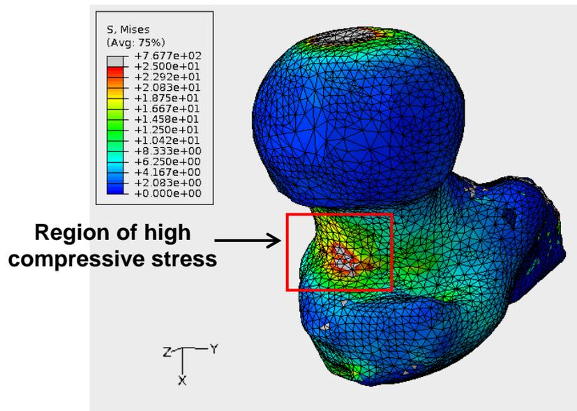
Figure 1. Local buckling of the elderly femoral neck by using Finite Element Method
