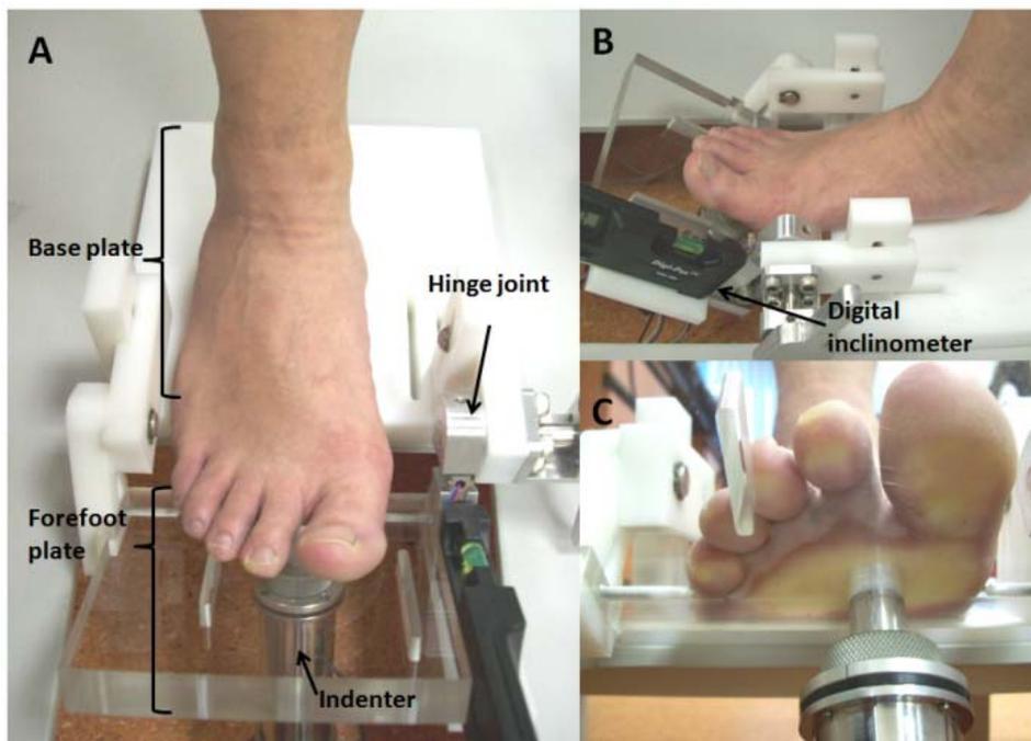
Figure 2. (A) Top view (B) side view (C) bottom view of experimental set up. The integrated indenter on the forefoot plate indents the plantar site and measures directly the force applied to the deformed tissue via a load cell mounted at the other end of the probe tip.
